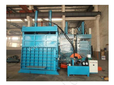
The long stroke baler machine is also popular as perfect OTR Tire baler (such as TBR vertical baler) and aluminum can baler. This vertical hydraulic press is designed for long stroke pressing , also with deep size chamber and known as Tire baling machine or can press.
